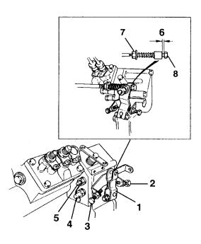
Fig. 92. Setting engine speed (RPM)
