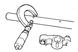
Fig. 26. Measuring of rocker shaft
