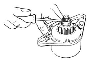
Fig. 119. Dismantling of the starter gear
