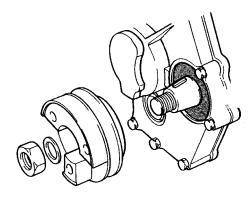
Fig. 56. Dismantling of crankshaft pulley
