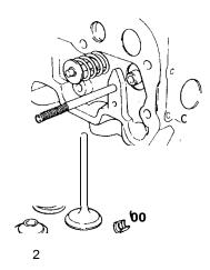
Fig. 29. Fitting of valves
