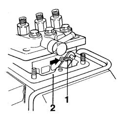
Fig. 65. Fitting of injector pump
