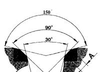
Fig. 20. Grinding of valve seat
