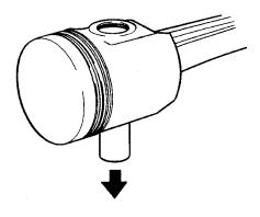
Fig. 40. Dismantling of gudgeon pin
