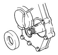
Fig. 54. Fitting of crankshaft seal
