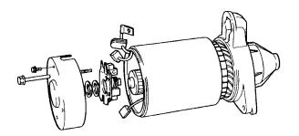
Fig. 116. Dismantling of the bearing shield
