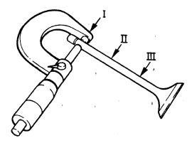
Fig. 18. Checking of valve spindle wear
