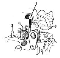
Fig. 13. Dismantling of rocker mechanism (MD2040)
