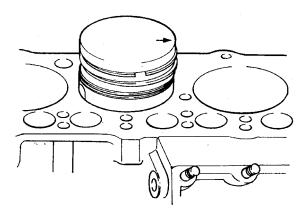
Fig. 39. Dismantling of piston
