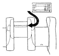
Fig. 78. Check measuring of measuring plastic
