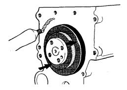
Fig. 81. Fitting of crankshaft seal
