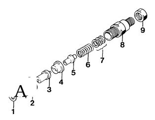
Fig. 103. Adjuster washers (7), injector
