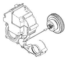
Fig. 64. Fitting of timing gear casing
