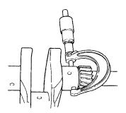
Fig. 74. Checking of bearing clearance
