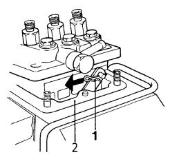
Fig. 57. Dismantling of injection pump
