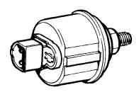
Fig. 125. Oil pressure sensor
