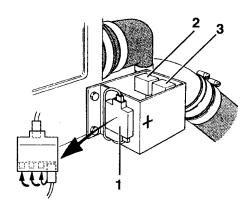
Fig. 121. Relay box with fuses
