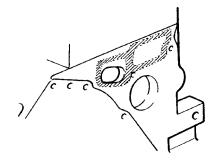
Fig. 108. Application of sealing compound (silicon)
