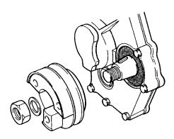
Fig. 55. Fitting of crankshaft pulley
