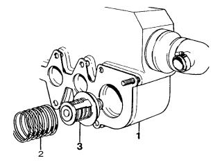
Fig. 9. Dismantling of expansion tank with heat exchanger
