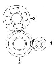
Fig. 58. Timing gears, basic setting
