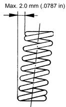
Fig. 23. Checking of linearity
