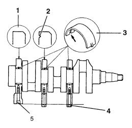
Fig. 79a. Fitting of main bearing cap MD2O10, MD2020, MD2030
