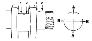
Fig. 72. Check measurement of crankshaft
