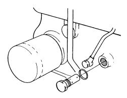
Fig. 83. Replacement of reducing valve
