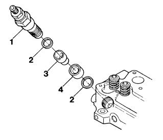
Fig.102. Dismantling of injector
