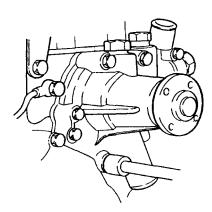
Fig. 11. Dismantling of circulation pump
