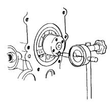
Fig. 80. Checking of axial clearance
