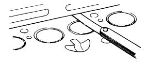
Fig. 15. Checking of cylinder head flatness
