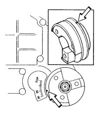
Fig. 90. Marking the pulley and engine block
