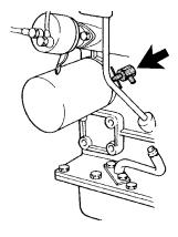
Fig. 105. Draining of the refrigerant
