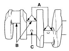
Fig. 73. Checking of recess radius
