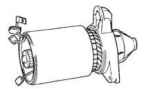
Fig. 117. Dismantling of the stator housing
