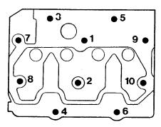
Fig. 30. Tightening diagram, MD2O10
