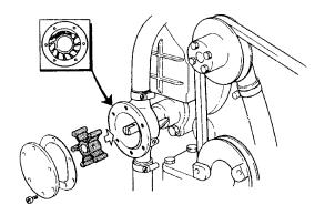
Fig. 109. Replacing the pump wheel
