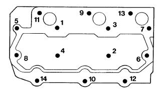
Fig. 31. Tightening diagram MD2020, MD2030, MD2040
