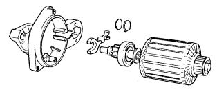
Fig. 118. Dismantling of the rotor
