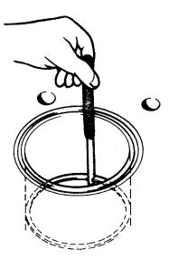
Fig. 41. Checking of piston ring gap
