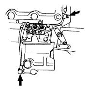
Fig. 33. Fitting of oil pressure pipe (cylinder block - cylinder head / rocker mechanism)
