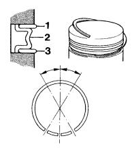
Fig. 52. Fitting of oil ring (MD2040)
