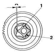
Fig. 84. Checking of oil pump clearance
