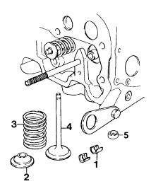
Fig. 14. Dismantling the valves
