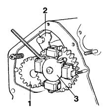
Fig. 67. Dismantling of camshaft
