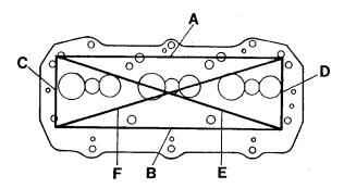
Fig. 16. Checking of cylinder head flatness
