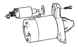
Fig. 115. Stripping of the starter motor
