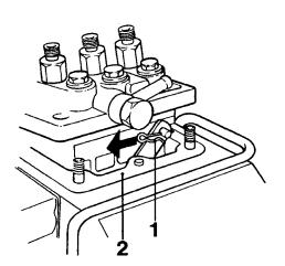
Fig. 87. Dismantling of the injection pump
