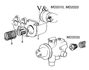
Fig. 35. Fitting of thermostat (MD2O10, MD2020, MD2030) and expansion tank.
