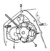
Fig. 70. Fitting the camshaft
