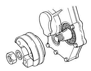
Fig. 66. Fitting of crankshaft pulley
