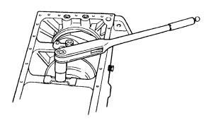
Fig. 71. Dismantling of main bearing cap
