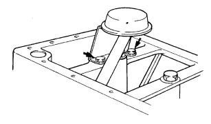
Fig. 38. Dismantling of oil strainer with induction manifold
