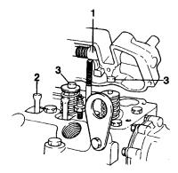
Fig. 32. Fitting of the rocker mechanism (MD2040)
