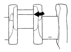
Fig. 77. Application of measuring plastic
