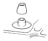
Fig. 28. Fitting of valve stem seals
