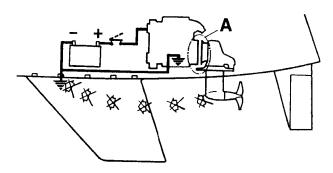
Fig. 113. Electrical insulation (A) of the flywheel housing and transmission
