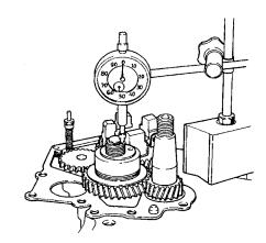
Fig. 63. Checking of oil pump's axial clearance
