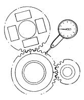
Fig. 60. Checking of gear flank clearance
