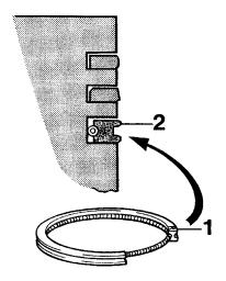
Fig. 51. Placement of piston rings
