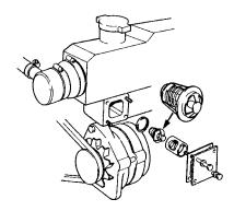
Fig. 36. Fitting of thermostat (MD2040)
