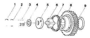
Fig. 62. Intermediate gear complete with oil pump
